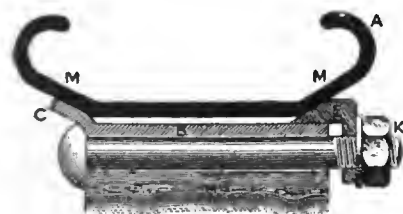
VINET RIM SECURED BY MOVABLE WEDGES.
